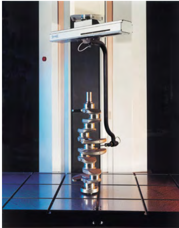
Figure 9 - Using a special drop-arm to measure a crankshaft.
