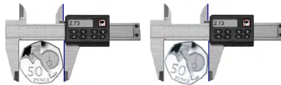
Figure 1 - Diameter measurement of a coin.
