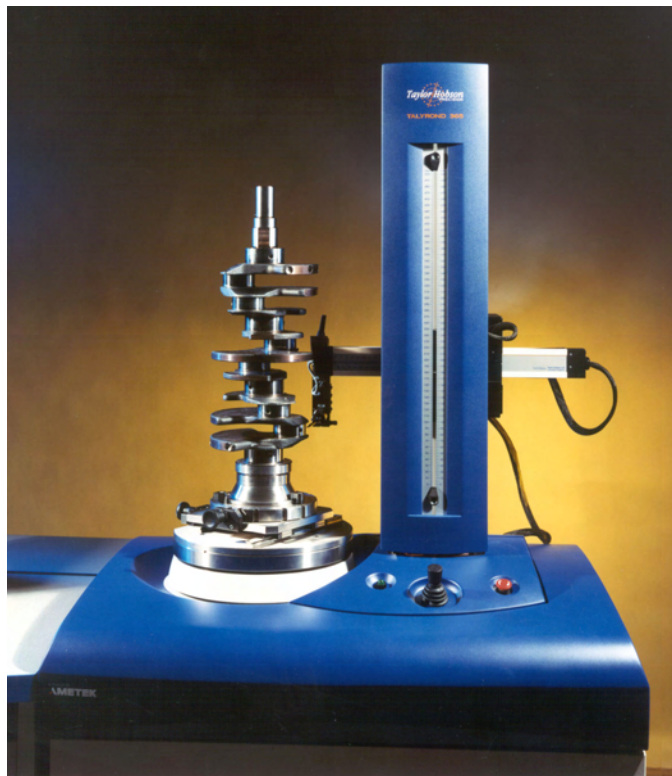
Figure 6 - An example of a rotating workpiece roundness measuring instrument.
