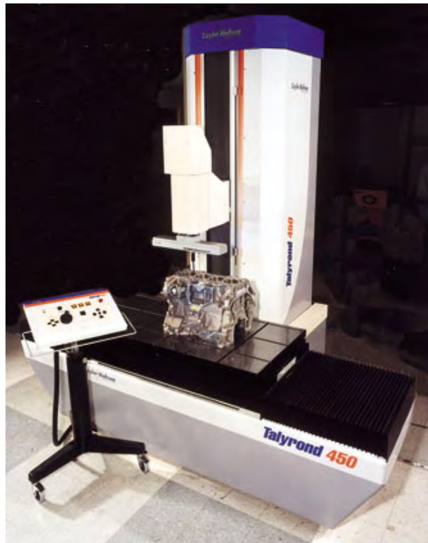
Figure 7 - A Talyrond 450 measuring an engine block.
