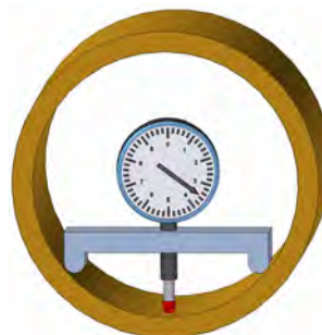
Figure 4 - Adaptation to measure large bores.
