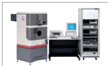
Interferometer as the standard for Gauge Block calibration (At Miyazaki Manufacturing Department)
