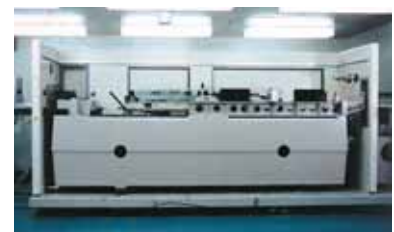
Interferometer as the standard for Linear Scale calibration (At Kiyohara Manufacturing Department)
