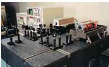
Iodine Absorption Stabilized He-Ne Laser as the standard for length measurement (At Tsukuba Calibration Center)
