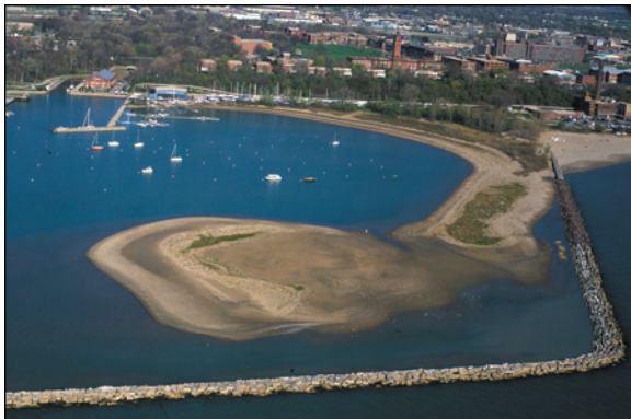
Oblique aerial photo of northern half of harbor viewed from the east showing close-up of sand accretion (May 3, 2000; photo by M. Chrzastowski, ISGS).
