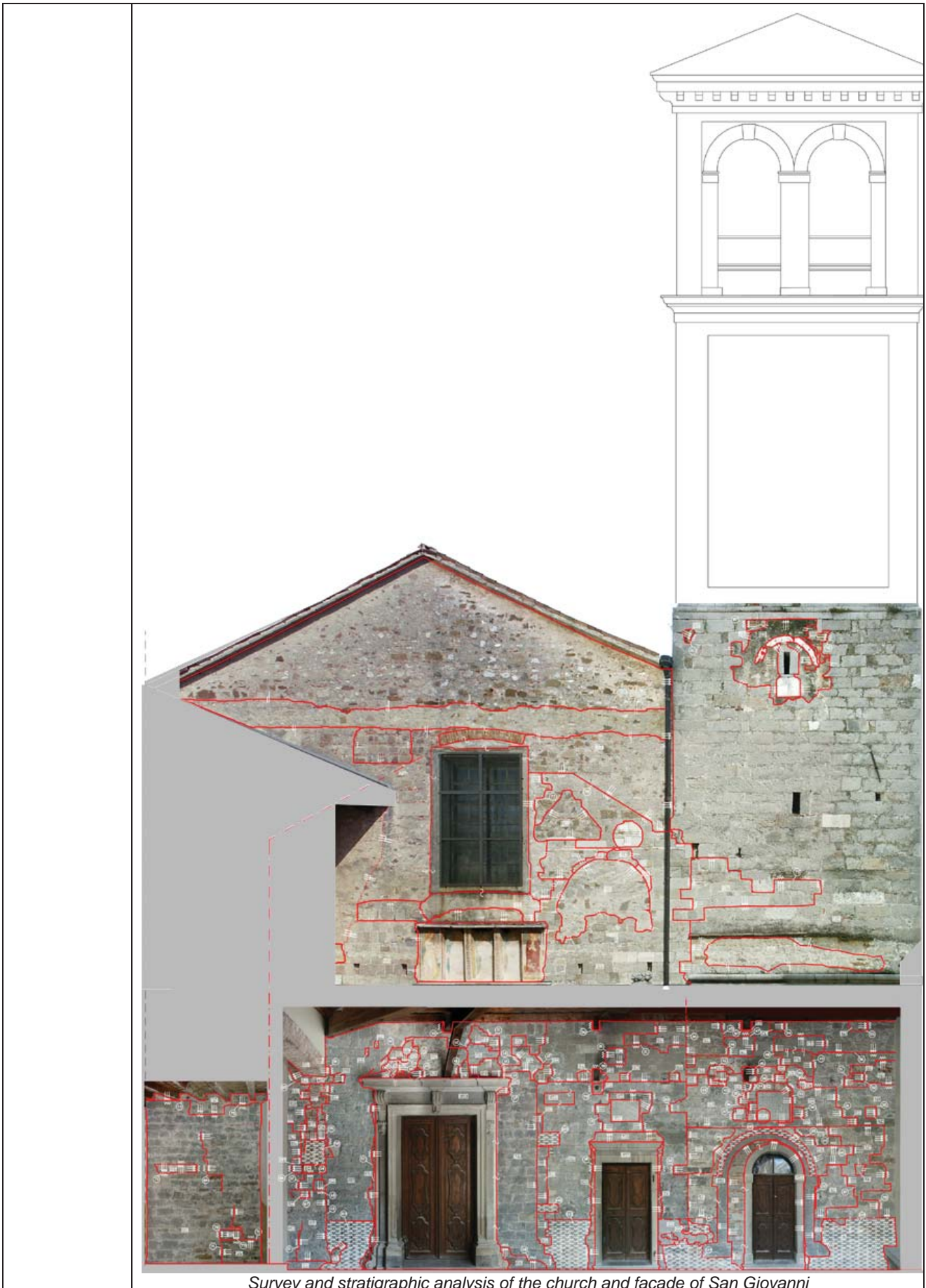
Survey and stratigraphic analysis of the church and façade of San Giovanni
