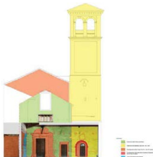
Study of the building phases of the Church based on the stratigraphic analysis UPGRADE OF THE WALKWAY BETWEEN THE COURTYARD OF SAN GIOVANNI AND THE
