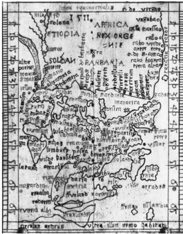
FIG. 10.14. MAP OF EUROPE AND NORTH AFRICA FOR USE WITH A SUNDIAL, DRAWN BY ERHARD ETZLAUB ON A "MERCATOR-LIKE" PROJECTION, 1511. The increasing spacing of the parallels of latitude toward the north pole (south is at the top) have led some authors to cite this map as a precursor to the Mercator projection, but because the map functioned as a sundial and not a map for the use of navigators, any direct link is unlikely.
