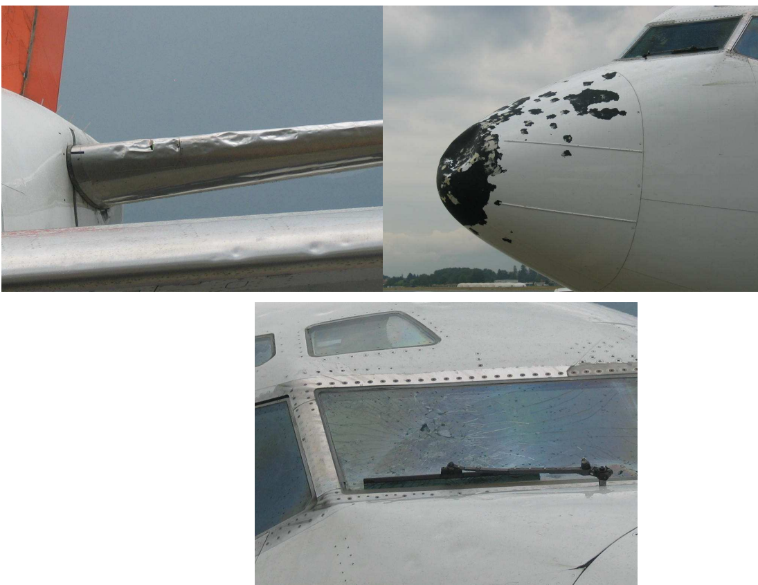
Figure 8.39 Hail damage to Boeing 737 aircraft
