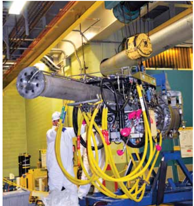
A worker inspects a fuelling machine at Bruce B.
