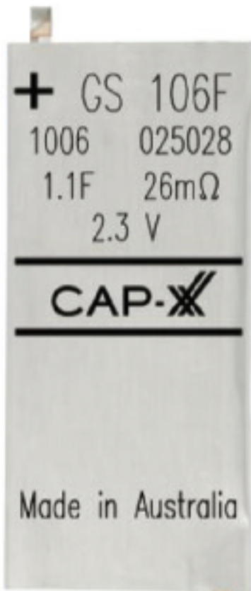
Figure 11 Australian Cap XX device. One of the smallest and most power components on the market.
