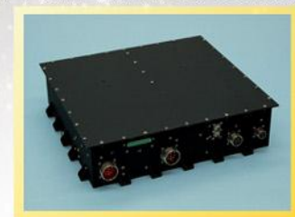
HALL THRUSTER PROPULSION SYSTEM 4.5 kW POWER PROCESSING UNIT
