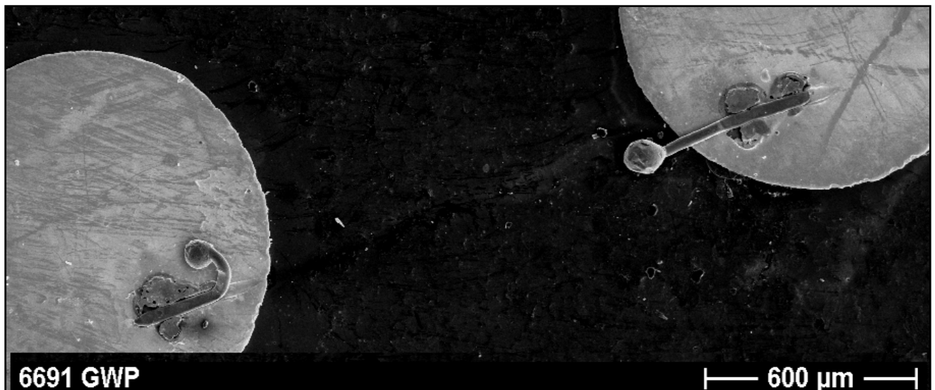
Figure 11: Molten filament (glow bridge) after.
