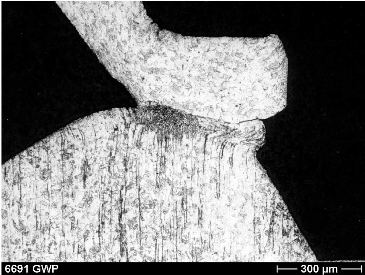
Figure 7: High quality condenser discharge welding of a membrane (above) with neck of calotte (above left) and support (below).
