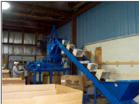
Figure 2: Plastic Housings at Shredder Line
