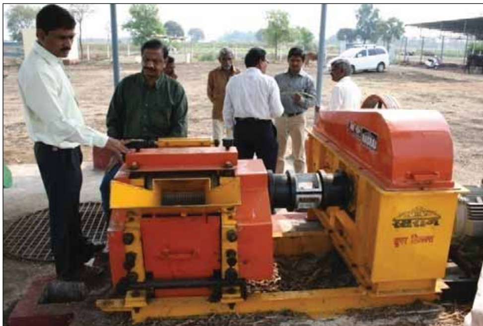
Fig. 8. The 3-roller 25 hp crusher.
