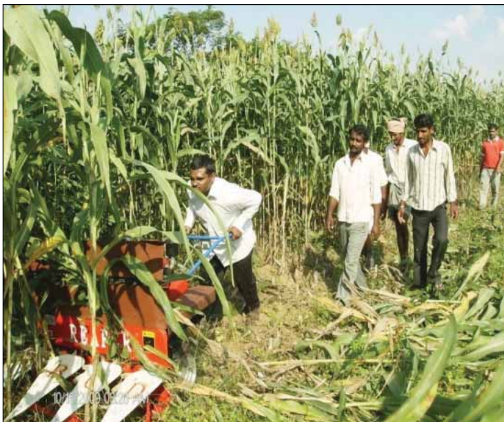
Fig. 6. Field testing of the modified reaper.
