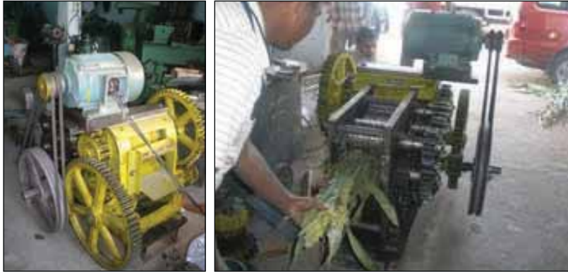
Fig. 7. The 3-pass 6-roller crusher and its testing.
