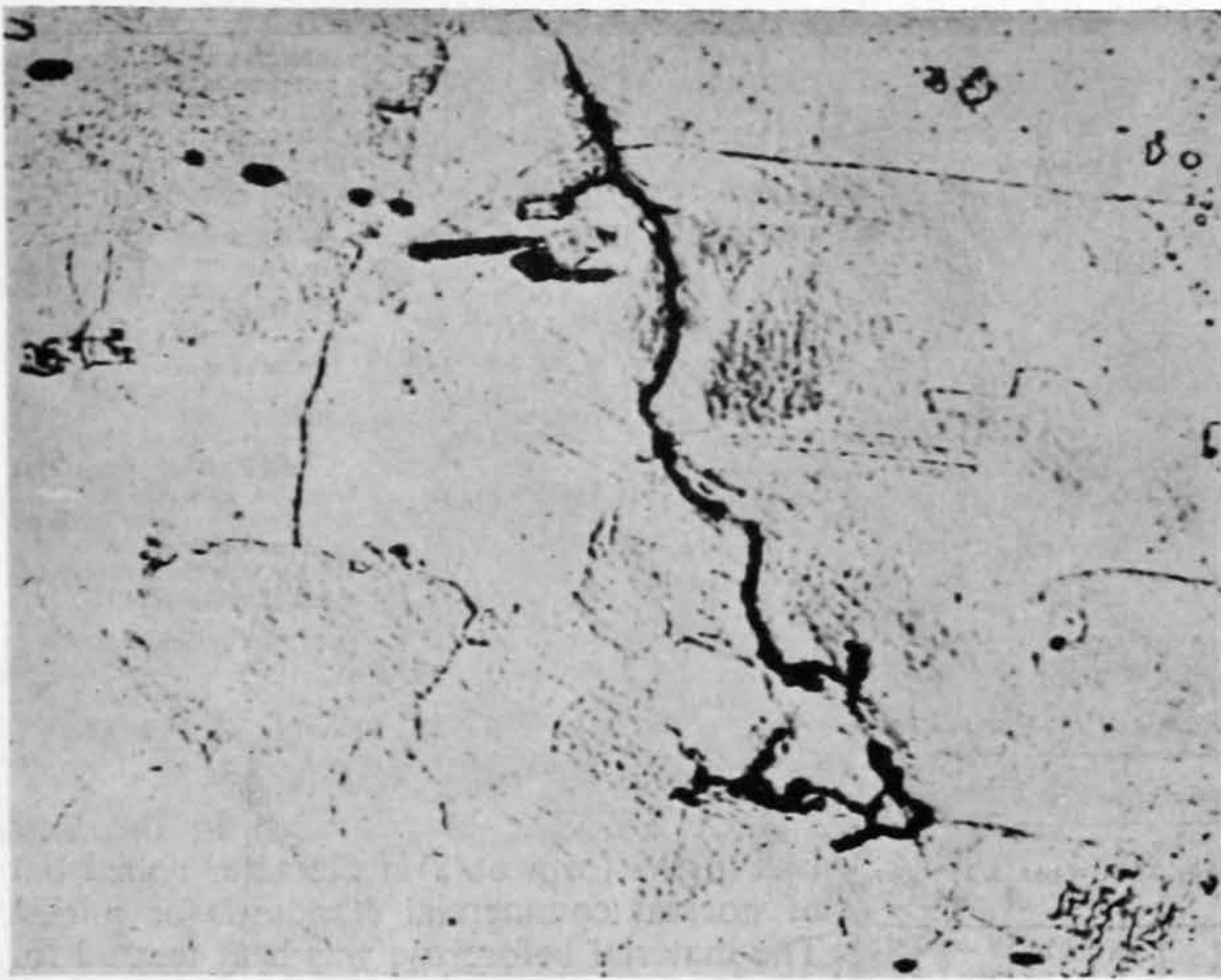
Fig. 18—Pure torsion stress 2 tons per square inch ; fractured, 5442 hours ; magnification \times 500
