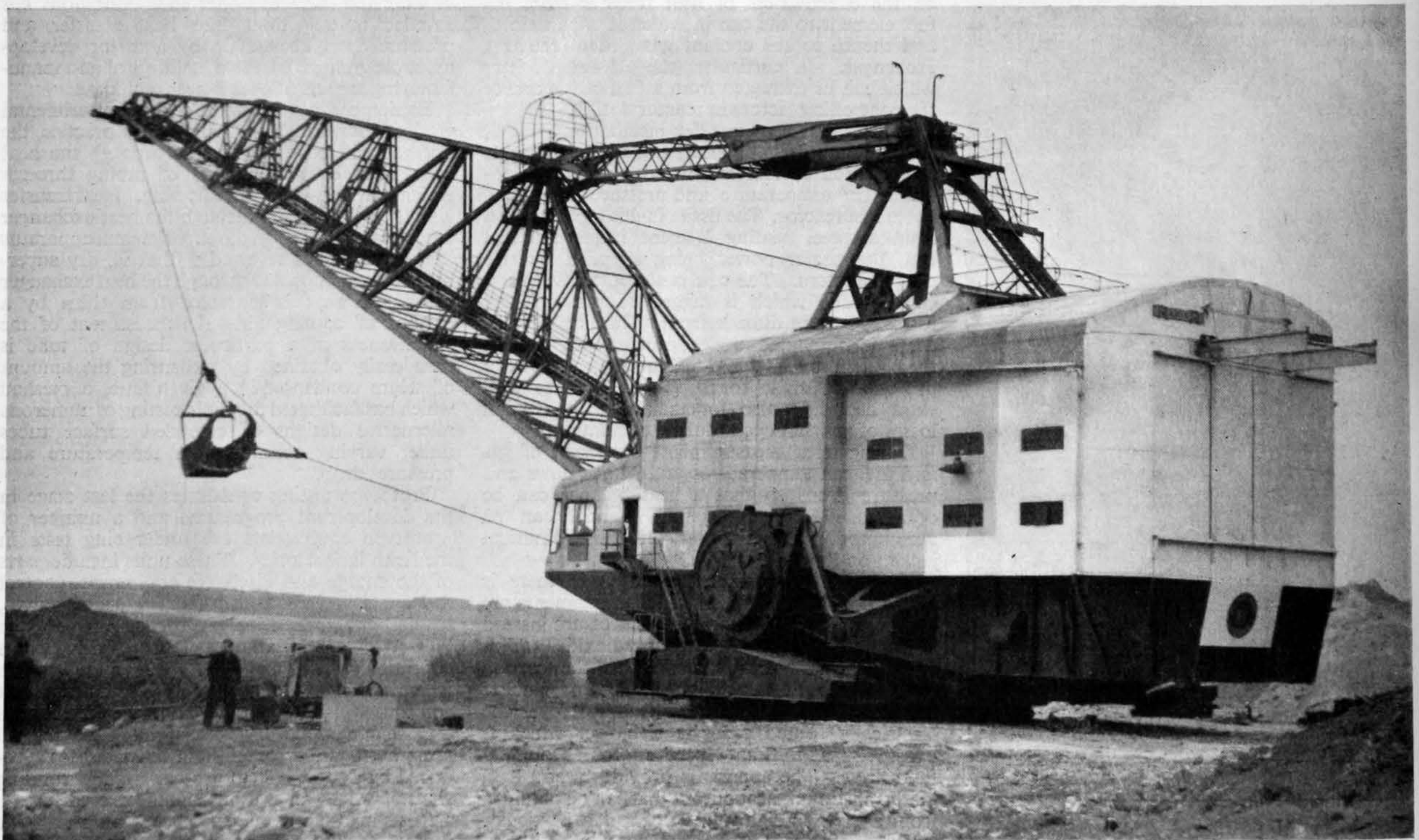
Walking dragline fitted with a 10 cubic yard bucket and arranged for a 184ft working radius
