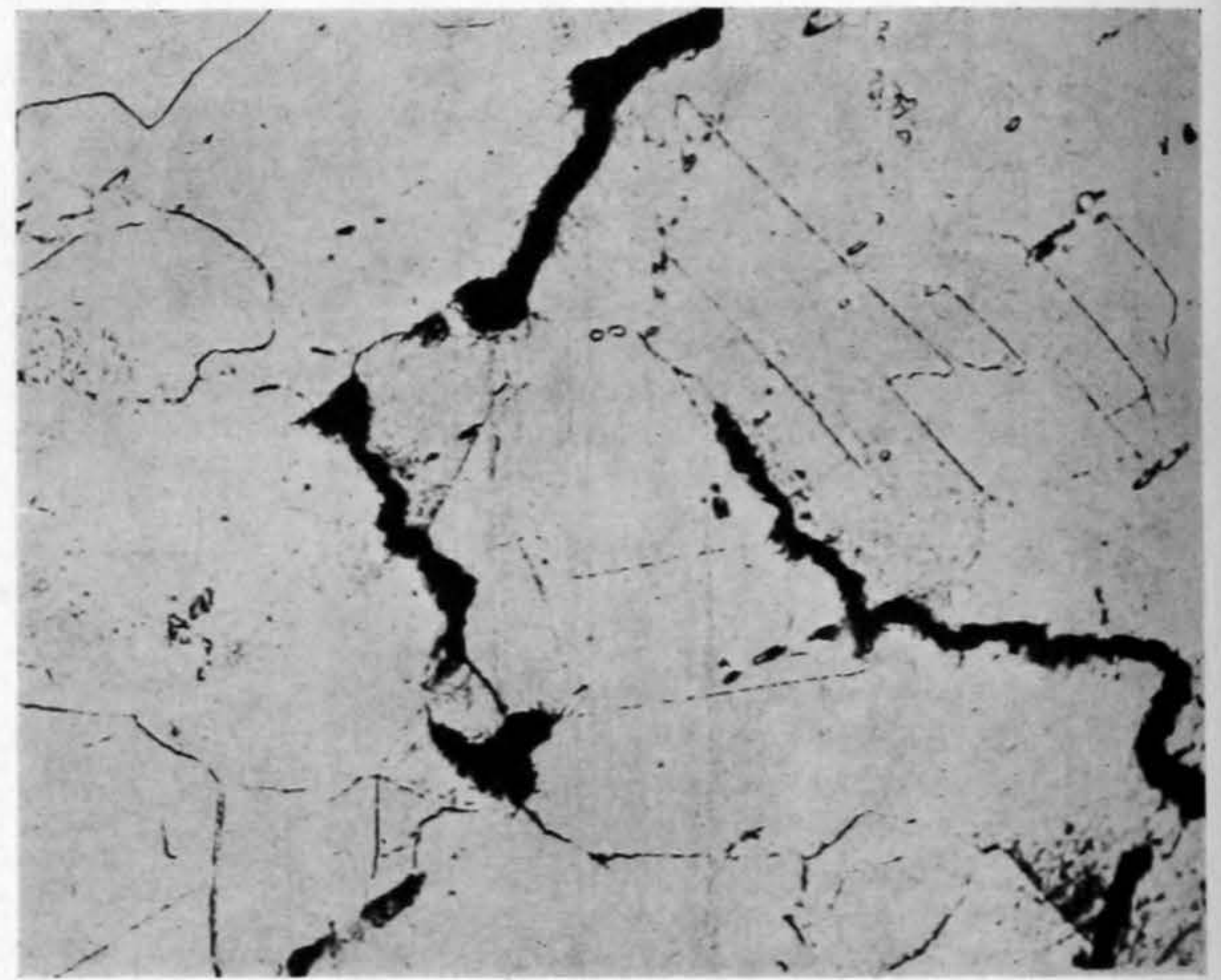
Fig. 21—Tension stress, 0.9 ton per square inch ; torsion stress, 2.25 tons per square inch ; fractured, 2082 hours ; magnification \times 500
