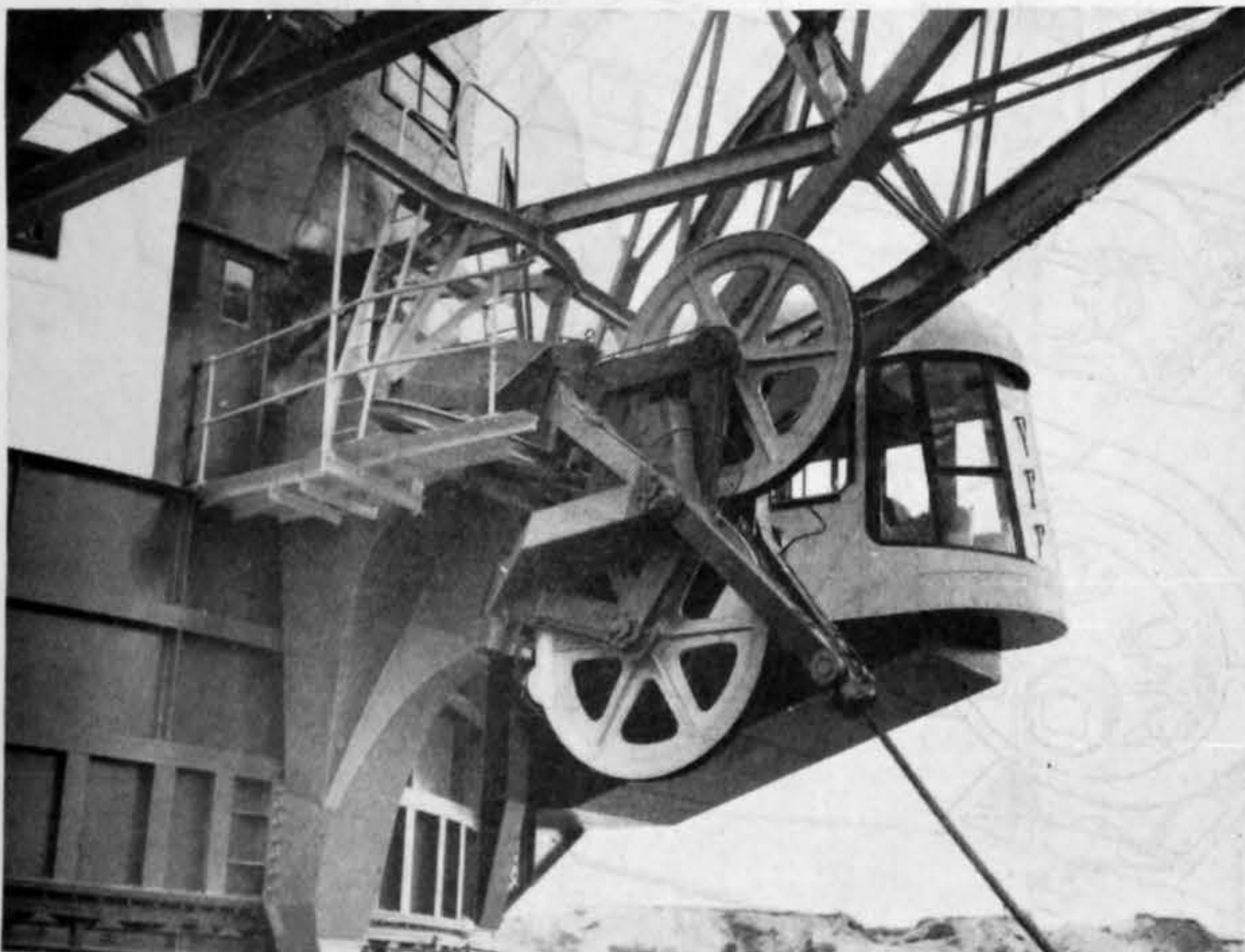
(Left) Foot of boom with drag gear. The driver's cab projecting beyond the machinery house at the side gives a clear view of all operations (Right) Head of boom suspension "A" frame. The legs of the boom suspension member have three sets of holes by the use of which the angle of the boom can be set at 25 deg., 30 deg. or 35 deg., to vary the capacity of the machine
