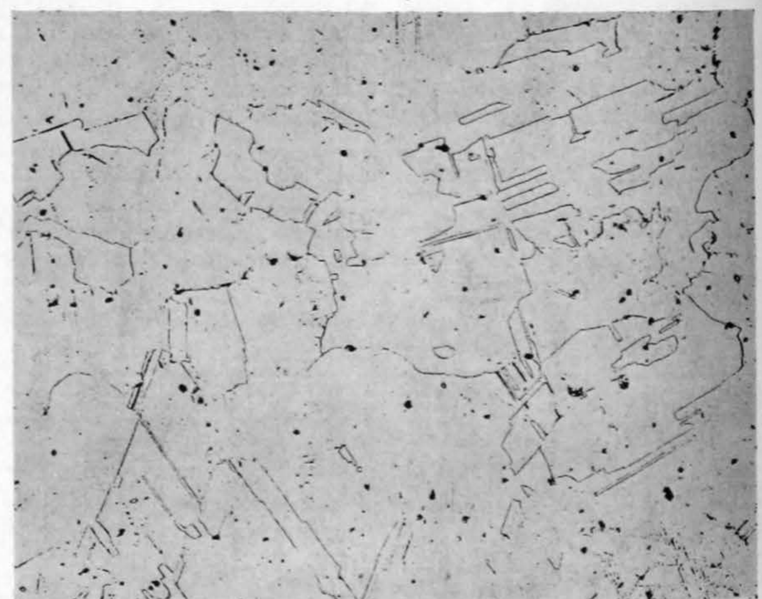
Fig. 23—Compression stress, 3 tons per square inch ; unbroken, 1250 hours ; magnification \times 200
