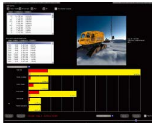
NVPerfHUD 4's Frame Profiler can identify the relative cost of each draw call in a frame and reports where it is bottlenecked.
