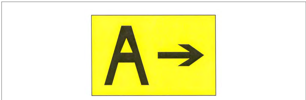
FIG 2-3-36 Direction Sign for Runway Exit
