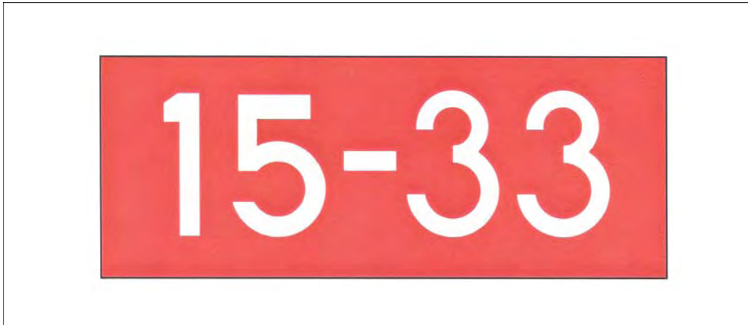
FIG 2-3-24 Runway Holding Position Sign
