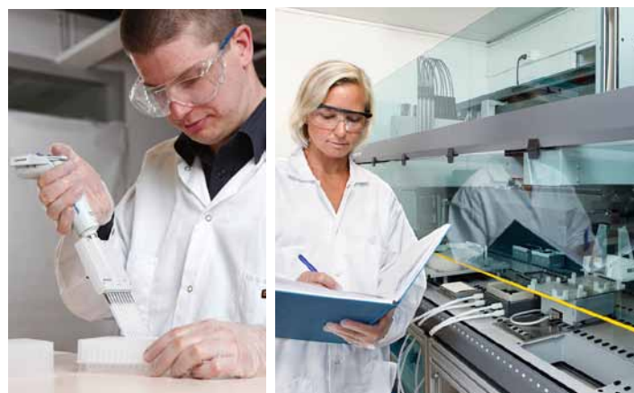
Fig 2. Manual or fully automated methods for high-throughput screening of CIP protocols. It is possible to do screening and optimization of CIP protocols manually, using multi-pipettes and manual centrifugation or vacuum filtration (left). The methodology can also be implemented on a fully automated system such as a Tecan robot (right).
