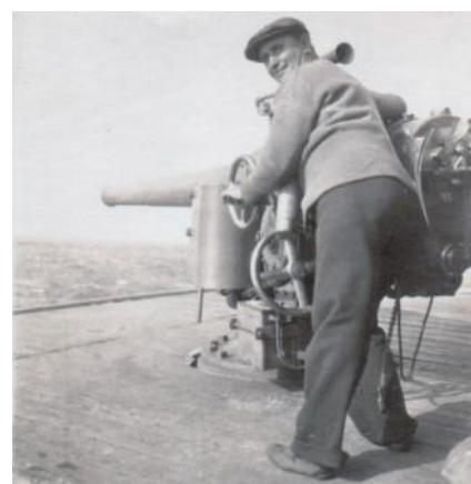
4.7-in QF gun mounted on a merchant vessel in WWI. The photo shows the low semi-circular shield fitted to these guns
