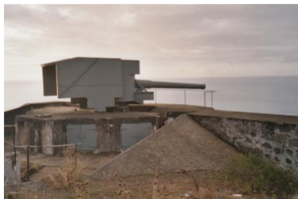
A 6-inch Mark 7 gun still in position on St Helena and showing the later WW2 period addition of a splinter shield
