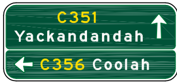
(a) On a wide list type ADS, e.g. Sign Nos G1-1, G1-2
