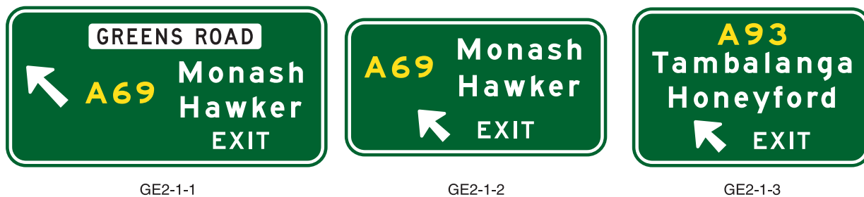
(a) Exit direction signs
