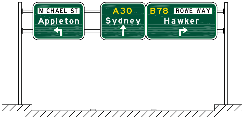
FIGURE 2.5 TYPICAL LANE DESIGNATION ASSEMBLY USING G9-7 SIGNS
