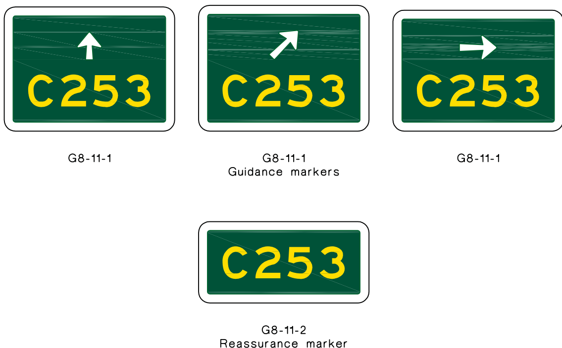
FIGURE 4.3 FREE STANDING GUIDANCE AND REASSURANCE MARKERS
