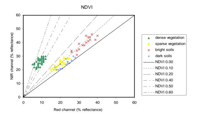
Figure 2: Scatter plot of Red and NIR channel values showing the NDVI isolines and different types of vegetation and bare soil values.
