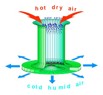
Figure 1 - Schematic description of the Energy Tower's operation
