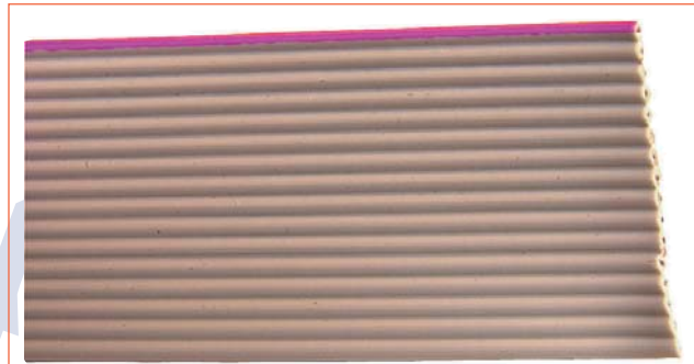
Here's what 16-way IDC ribbon cable looks like. The insulation is all the same colour, but there's a coloured stripe down one side.
