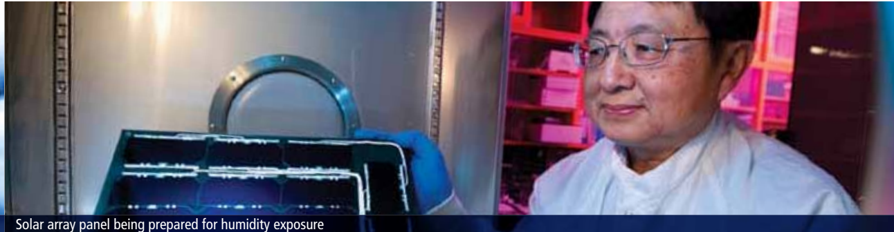
Solar array panel being prepared for humidity exposure
