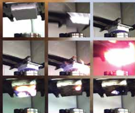
Sequence of images from insulation flame test
