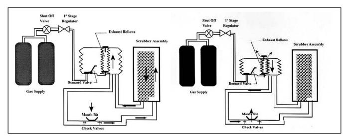
Figure 25. Schematics of the bellows-in-bellows action of dual-bellows VVE rebreathers. The exhalation phase is shown in the left panel, and inhalation is shown in the right panel.
