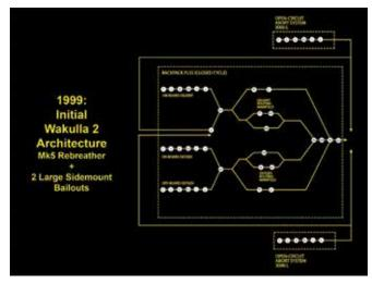
Figure 11. A fault-tree diagram for a partially redundant rebreather designed for the Wakulla 2 project in 1998. The system used dual gas supplies routed to a single rebreather with a manual backup control system.
