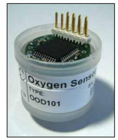
Figure 5. Prototype of our "smart" galvanic  $O_2$  sensor.
