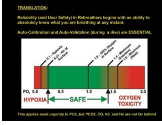
Figure 30. Rebreathers actively control the partial pressure of oxygen in the breathing loop, and it must be maintained in a survivable zone. Oxygen sensors provide the critical information to an onboard electronics system that controls  $PO_2$ . But sensors can age, change readings at different temperatures and pressures and can do so during the course of a dive. The only means to safely deal with that is to validate these sensors during the dive.
