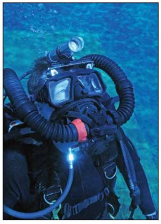
Kirby Morgan M-48 Mod -1 mask with open-circuit switch-over pod. Photo courtesy Dive Lab.
