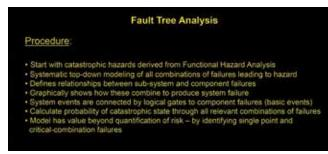
Figure 7. Fault-tree analysis: A numerical probability method for assessing the likelihood of failure of a system in which the components are ascribed individual failure probabilities. It is a useful tool for quantitative comparison between competing system designs.
