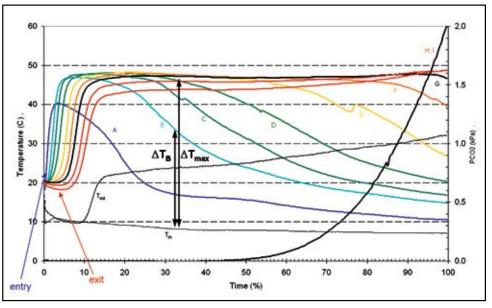
Figure 8. Temperature variations recorded from nine sensors placed in a  $CO_2$  scrubber and the  $CO_2$  in the inspiratory hose. Temperatures are shown on the left vertical axis and  $CO_2$  level on the right vertical axis. Time is expressed as a percentage of the entire run; 100 percent does not mean the time to a physiologically acceptable  $CO_2$  level.
