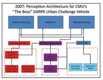
Figure 38. Perception architecture for an unmanned ground vehicle.
