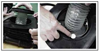
Figure 27. Oxymix 3C inner (exhaust) and outer bellows (left and right panel). The demand valve actuator is pointed out in the right panel. U.S. Navy photo.
