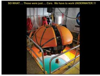
Figure 40. The DEPTHX underwater vehicle successor, known as ENDURANCE, preparing for a 10-hour subice mission in Antarctica. The vehicle can explore, map, and navigate on its own in 3D with only limited goal state programming.
