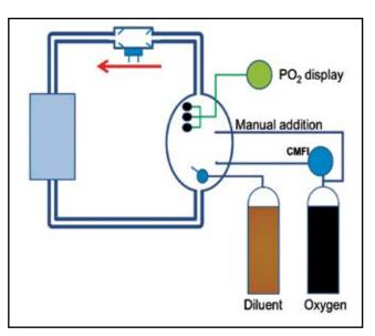
Figure 6. Simplified and stylized depiction of an mCCR. See text for explanation. Note that the oxygen cells are depicted as being sited in the counterlung, but this is never the case. A manual injector for diluent gas has been omitted for simplicity. CMFI = constant mass flow injector.
