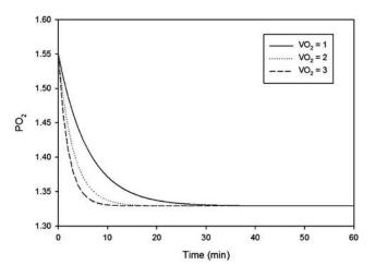
Figure 26. VVE rebreather PO<sub>2</sub> control for three levels of oxygen consumption and three RMVs. John R. Clarke figure.
