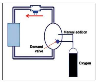
Figure 3. Simplified and stylized depiction of a pure oxygen rebreather. See text for explanation. Some of these devices also have a CMF injector.
