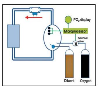
Figure 5. Simplified and stylized depiction of an eCCR. See text for explanation. Manual injectors for both oxygen and the diluent gas have been omitted for simplicity.
