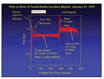
Figure 51. Typical base-level stored data from the Mk5 rebreather:  $PO_2$  versus time.
