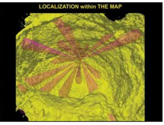
Figure 42. A data replay frame from a DEPTHX mission to Cenote Zacaton. The yellow faceted surface represents the map of Zacaton created by DEPTHX while exploring downward. The red beams represent tight beam sonar pings. The system uses these to estimate its current position within the map.
