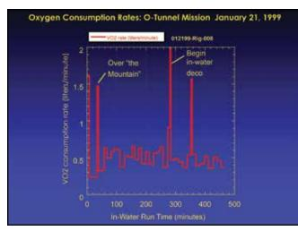
Figure 53. Typical derived data from the Mk5 rebreather:  $VO_2^*$  (oxygen consumption rate) versus time.
