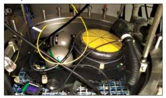
Figure 2b. Mk 16 closed-circuit rebreather in ANSTI test chamber. Photo courtesy Dive Lab.
