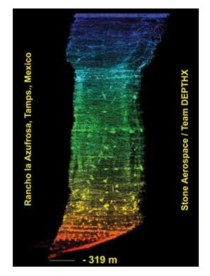
Figure 43 (version v2). Profile map of Cenote Zacaton created by DEPTHX. Green points above the water surface (blue) are from surface-based 3D LADAR data. Bottom breakdown pile slope is in red, and the image is looking into the narrow (90 m [295 ft] wide) view; the long axis (into the page) width is 140 m (459 ft). Total depth of the geological feature is 335 m (1,099 ft).
