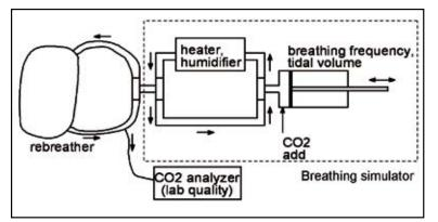
Figure 1. Schematic of the test set-up for determining the endurance of a  $CO_2$  scrubber. The rebreather to be tested is on the left. The interrupted line encloses the parts of the breathing simulator. Arrows indicate the piston movement and gas movement, respectively.
