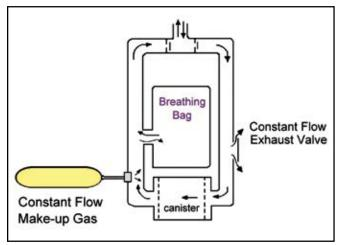
Figure 3. Schematic of the simplest mechanical semiclosed-circuit rebreather.
