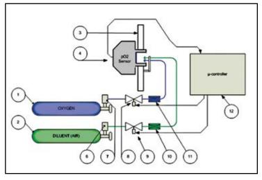
Figure 3. Schematic of our true PO<sub>2</sub> sensor signal validation system (1: O<sub>2</sub> tank; 2: diluent tank; 3: sensor support; 4: PO<sub>2</sub> sensor; 6,7: pressure regulators; 8,9: solenoids; 10,11: flow restriction orifices; 12: microcontroller). Reprinted with permission of Diving and Hyperbaric Medicine (Sieber et al., 2008).
