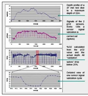
Figure 4. Data from a 100-minute test dive (6,000 seconds) in the Mediterranean Sea to a maximum depth of 22 m (72 ft). (A: depth profile; B:  $PO_2$ sensor signals of two sensors; C: calculated  $fO_2$ ; D: one validation cycle) Reprinted with permission of Diving and Hyperbaric Medicine (Sieber et al., 2008).
