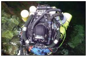
Figure 2. Cave diver Sandy Varin, in the entrance to the Pearse resurgence in NZ, wears a twin rebreather system built by combining a backmounted rEVO unit with a Classic Inspiration scrubber and circuit attached to the diver's left side. Photo by Richard Harris.
