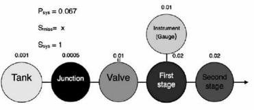
Figure 2. Probability failure tree for a standard open-circuit scuba system.
