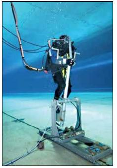
Figure 2. Controlled manned testing in a dive tank using a cycle ergometer.
