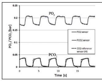
Figure 9: Sample breath-by-breath recording of  $PO_2$  and  $PCO_2$  from the transducer module in the rebreather mouthpiece. Reprinted with permission of Diving and Hyperbaric Medicine (Sieber et al., 2011).
