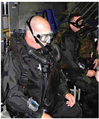
Figure 14. Divex Shadow Excursion diver instrumented with an oxygen sensor and data recorder. Photo by John R. Clarke.
