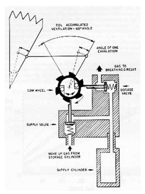
Figure 21. Interspiro ACSC ventilation control mechanism.
