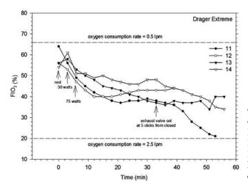
Figure 13. Effect of exhaust valve positioning on the bag oxygen concentration due to lack of activation of the demand-activated fresh gas add valve. John R. Clarke figure.
