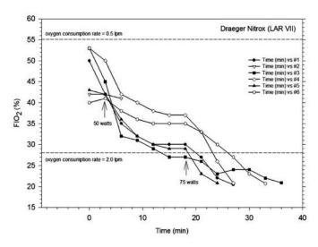
Figure 12. Response of a CMI rebreather to divers with unexpectedly high oxygen consumption rates. John R. Clarke figure.
