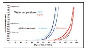
Figure 5. Reduction in absorbent canister endurance with a  $10^{\circ}$ C ( $50^{\circ}$ F) reduction in water temperature; n=3 runs at each temperature.
