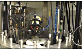
Figure 2a. Open-circuit band mask in ANSTI test chamber. Photo courtesy Dive Lab.
