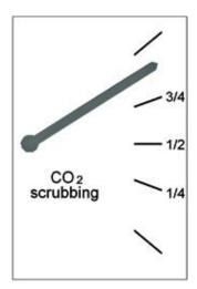
Figure 6. Illustration of an ideal scrubber gauge.
