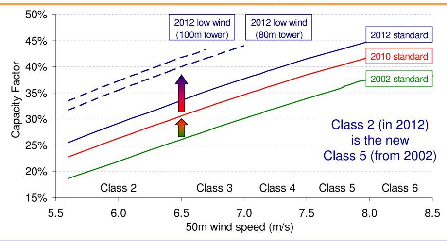
Modeled capacity factor improvement driven by larger rotor swept area in proportion to nameplate capacity, as well as higher hub heights; increase is especially apparent with newest batch of low-wind-speed turbines
