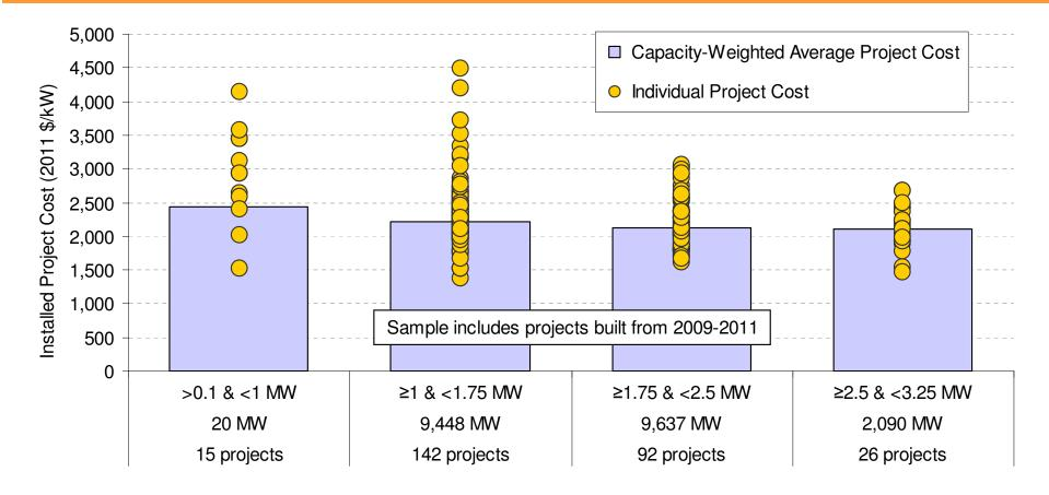
**Theory:** A project may be built less-expensively using fewer larger turbines instead of a larger number of smaller turbines
