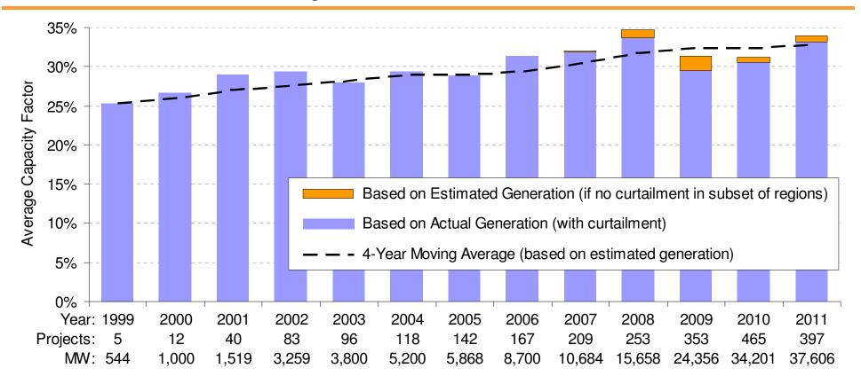
Capacity factor increase is less than what might be expected based on turbine scaling and other design improvements
