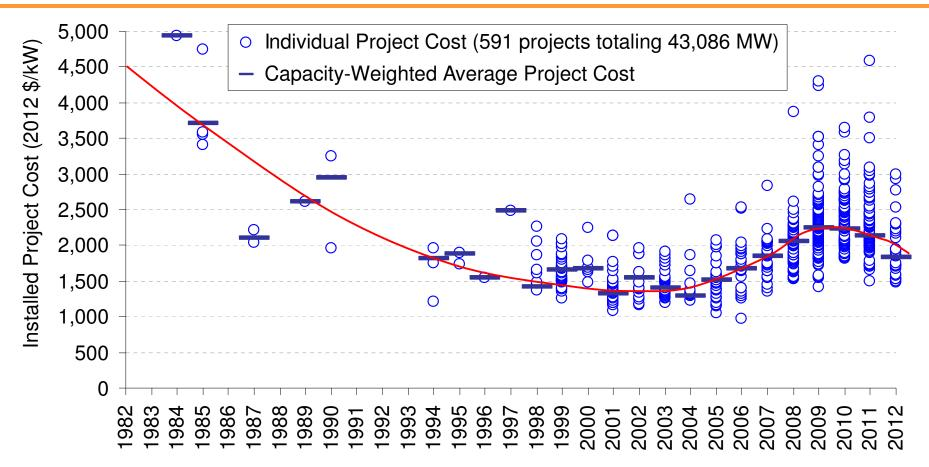
A preliminary sample of ~3 GW of 2012 projects shows estimated installed costs of around \$1,830/kW on average
