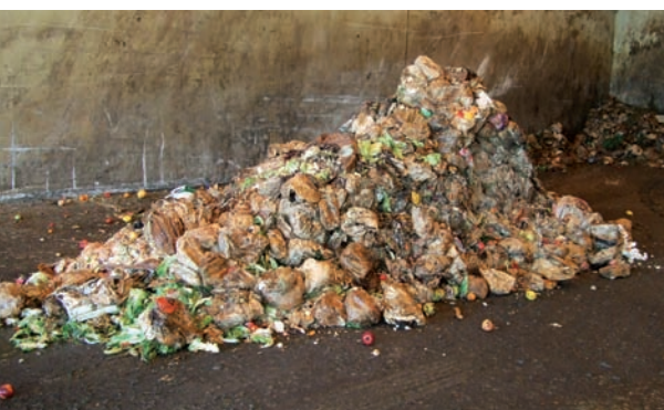
Photo 1. Source separated household waste to be used as substrate for biogas production. The composition of biogas is depending on the type of substrates used in the digestion.
