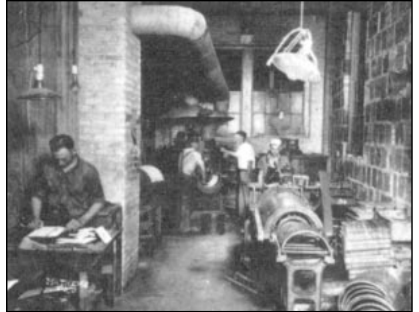
In 1921, the Times bought a Hoe press (left), capable of printing a 24-page paper. In the stereo room (above), curved metal casts of pages were made and locked onto the press.
