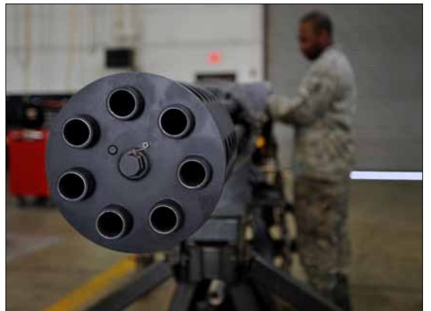
Staff Sgt. Michael Greer, 51st Munitions Squadron aircraft armament systems and weapons technician, services an A-10 Thunderbolt's 30-mm gun at Osan Air Base, Republic of Korea, Sept. 25, 2013. The A-10's gun is capable of firing 3,900 rounds per minute to defeat a wide variety of targets, including tanks.
