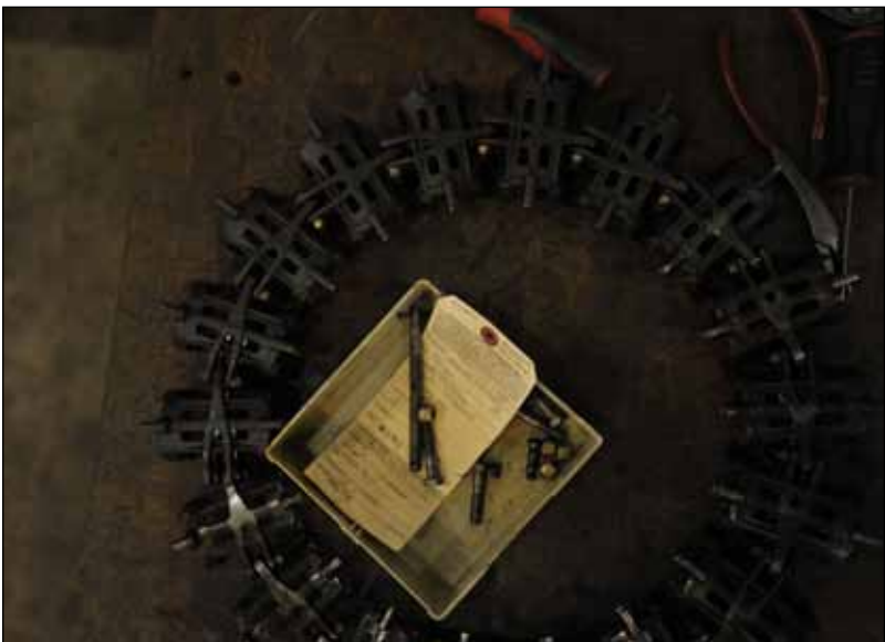
An element from an A-10 Thunderbolt's ammunition feeder awaits maintenance at Osan Air Base, Republic of Korea, Sept. 25, 2013. Technicians in the weapons back shop perform scheduled and unscheduled maintenance tasks to A-10 and F-16 Fighting Falcon weapons systems in proper working order.
