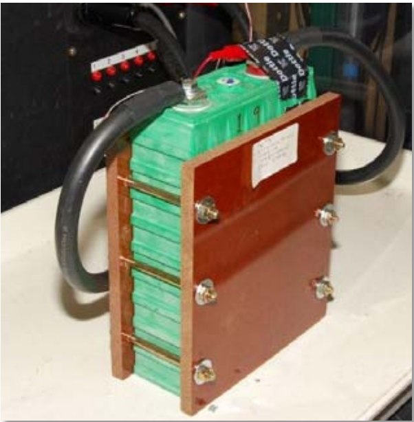
International battery Li-ion FePO 4 large format prismatic 160 Ah cells
