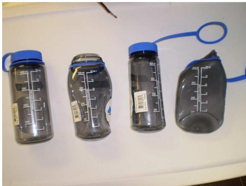
**Figure 17:** Heat Treated Tritan™ Copolyester Bottles. **1:** New Tritan™ copolyester bottle. **2:** After 1 hour ramping from 25 to 125 °C. **3:** 2 hours in autoclave at 102 °C. **4:** 2 hours in autoclave at 121 °C. This sample has turned opaque which is an indication that crystallites have formed.
