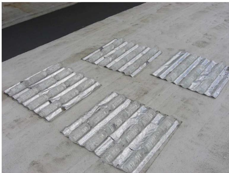
**Figure 8:** Solar Exposure of PETE Bottles: Bottles were exposed to sunlight on the roof of Kelley Engineering Center for 3 months. The bottles were placed on corrugated PVC material wrapped in aluminum foil.
