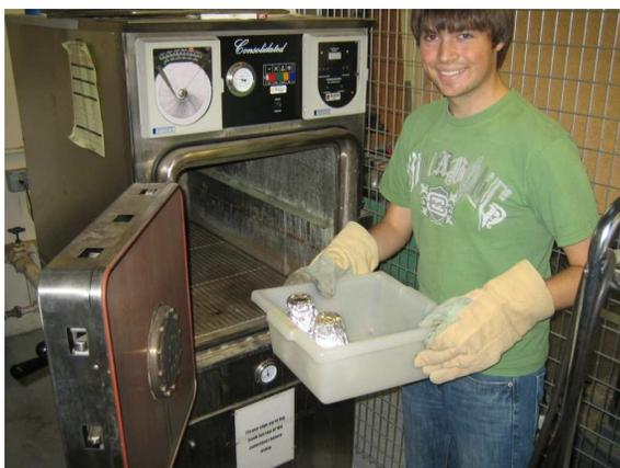
**Figure 7:** Autoclaving Polycarbonate Bottles
