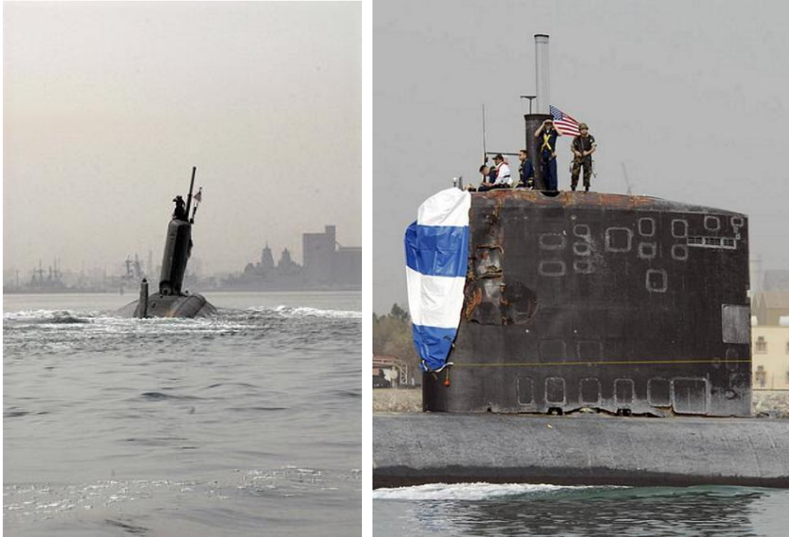
Figure 32. The collision of the Hartford with the New Orleans on March 20, 2009 caused damage to its communication gear and bent its sail.
