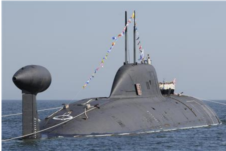
Figure 30. Akula Class Russian nuclear submarine with its tail sonar gear.
