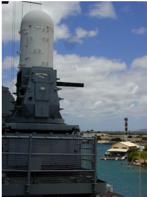
Figure 12. The Phalanx radar-guided gun, nicknamed as R2-D2 from the Star-Wars movies, is used for close-in ship defense. The radar controlled Gatling gun turret shooting tungsten armor-piercing, explosive, or possibly depleted uranium munitions on the USS Missouri, Pearl Harbor, Hawaii. Photo: M. Ragheb.
