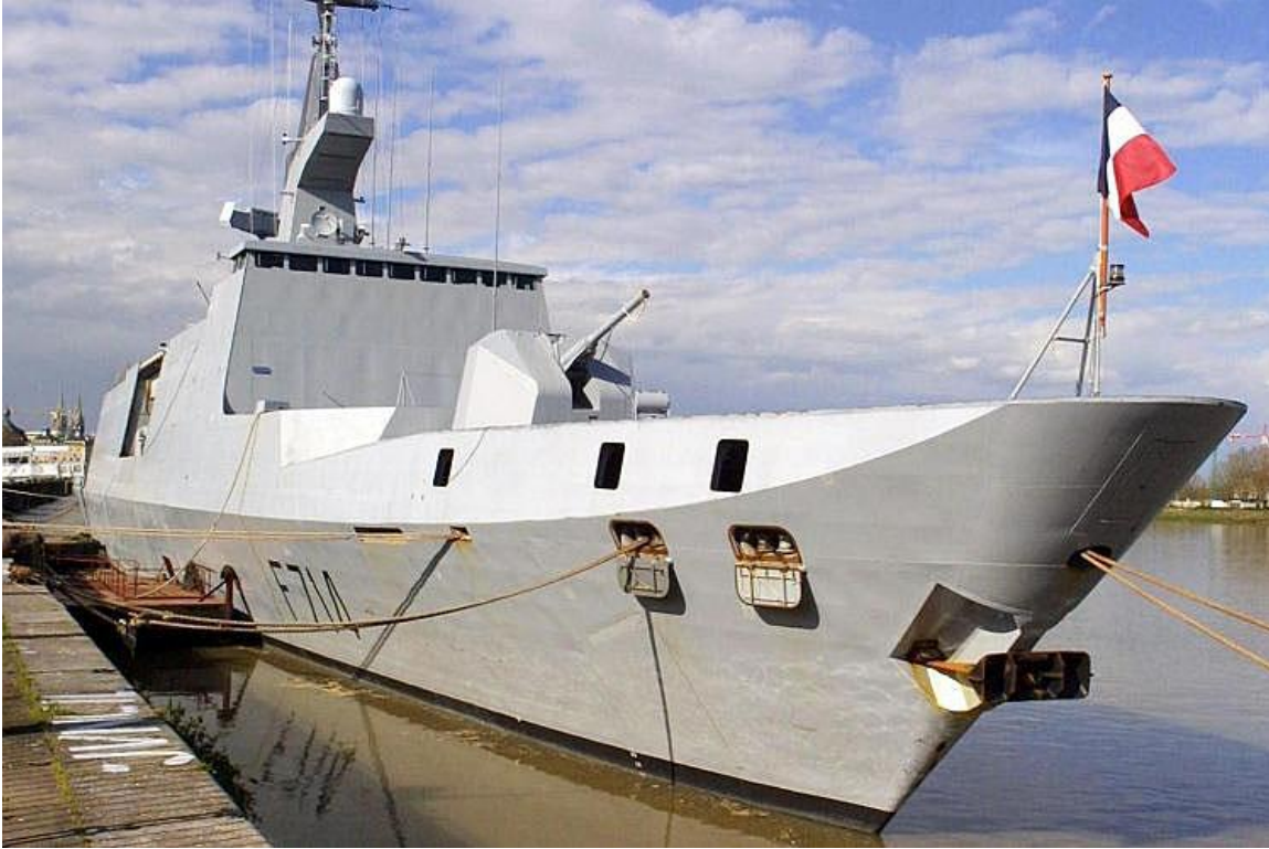
Figure 36. Stealth radar deflecting technology implemented into a French Lafayette class frigate, 2001.
