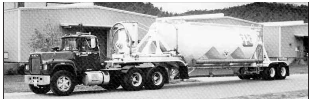
Pressure differential hopper trailer for delivery of PELS caustic soda beads in bulk.
