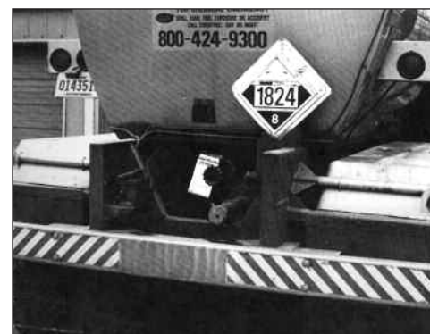
Hoses, valve and unloading connection at rear of tank truck.
