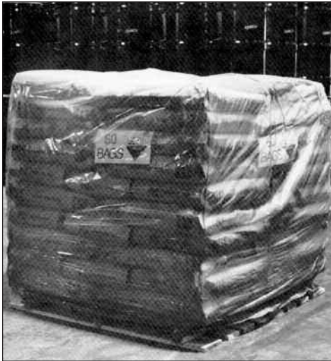
The entire pallet load, (foreground) 1 1/2 tons, consisting of sixty 50-pound bags, is protected by a shrink-wrapped polyethylene film. PELS Caustic Soda beads are also packaged in steel and fiber drums (background).
