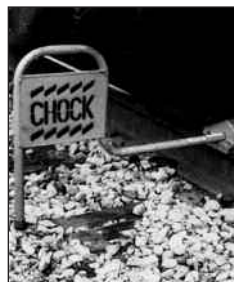
Wheel chock for tank car.
