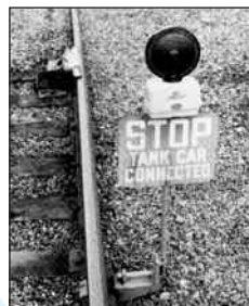
Derail. Stop sign stands between tracks.
