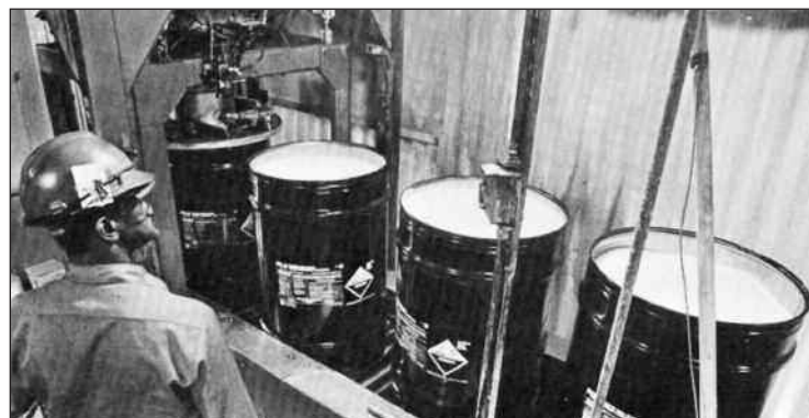
Drumming PELS caustic soda beads.
