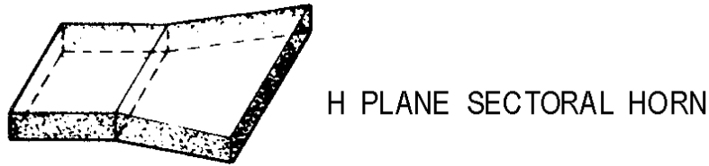
Figure 1-44B.—Waveguide horns. H PLANE SECTORAL HORN.
