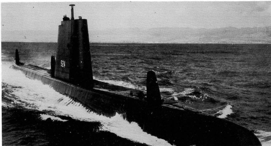
Submarine installation included passive sonar arrays inside the three fin-shaped sonar domes using length of the vessel as baseline for the complete receiving array.
