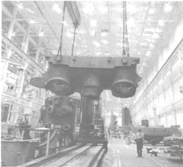
Interior view of the #1 Shop (Heavy Manufacturing) showing one of the many overhead bridge cranes which featured radio or pendant controlling with capacities ranging from 3 tons up to 350 tons.
