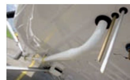
ENGINE OIL DRAINING SYSTEM
