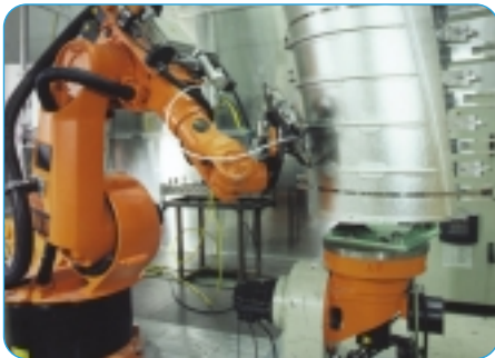
Protecting the environment. Development of the laser welding process for aluminium materials to replace conventional machining and riveting technology, which weakens materials and produces metal waste
