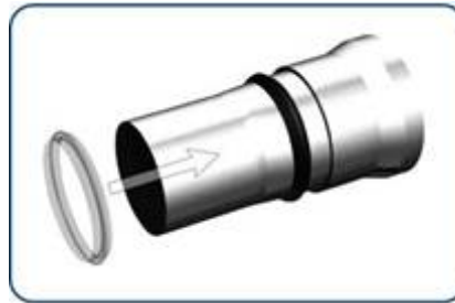
2. The gasket is loaded onto a mandrel
