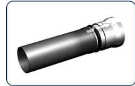
3. The pipe is formed over the mandrel
