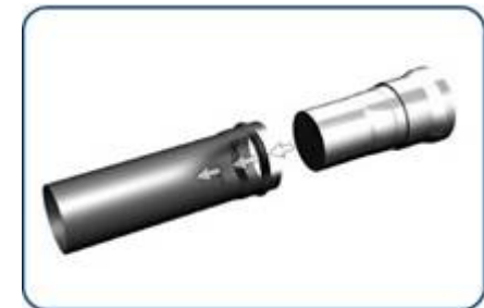
6. The pipe is pulled off the mandrel
