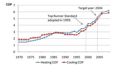
Figure 3. Long term trend of energy efficiency of room air conditioners
