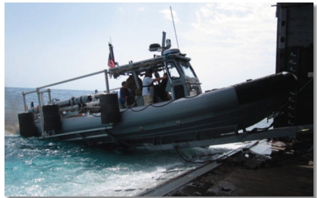
Figure 10. Mk 18 Mod 2 11-m RHIB stern gate launch and recovery system.
