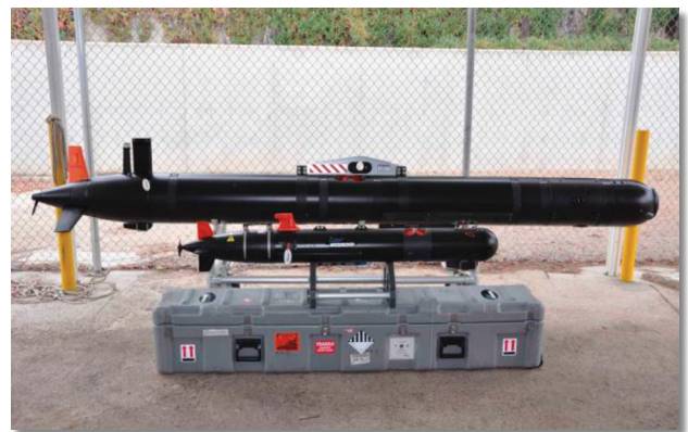
Figure 2. Mk 18 Mod 1 and Mod 2 UUVs. (Image courtesy of Space and Naval Warfare System Center, Pacific.)
