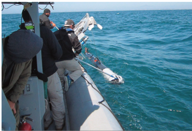
Figure 13. Civilian crew recovering UUV in 11-m RHIB with forward-looking sonar module.
