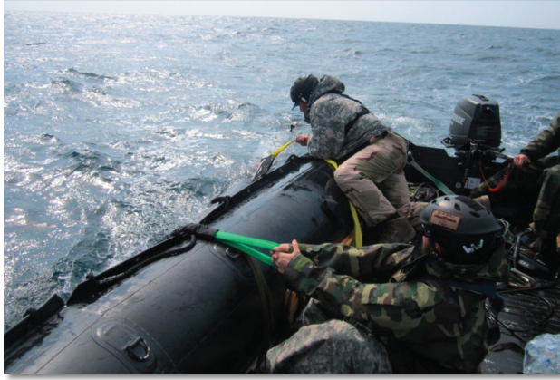
Figure 12. Civilian crew recovers Mk 18 Mod 2 UUV in CRRC during overseas sensor testing.
