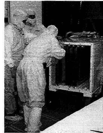
Figure 12. The blastshield transfer box is used for ammonia curing of sol gel coated glass and for clean storage of assembled units.
