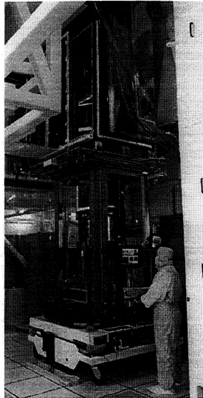
Figure 15. This slab cassette transfer vehicle was used for system development and AMPLAB operation.
