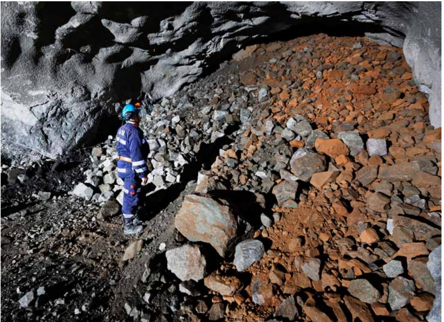
LKAB has developed effective methods for extracting residual ore from older production drifts. Roger Niemi, head safety officer, makes an inspection before unloading begins.
