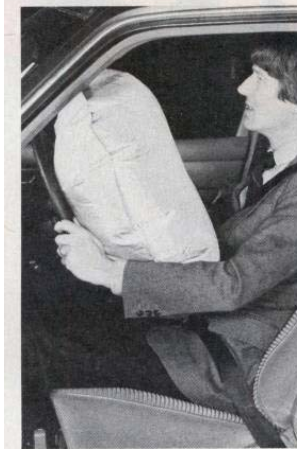
Chest-protecting air bag inflates from the steering wheel in 1/20 of a second, preventing injury as the driver is thrown forward. After driver hits it, the bag deflates.
