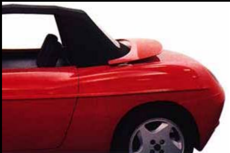
One idea that never took place. Spoiler set and use as a lid when the hood is open. (March 1992)
