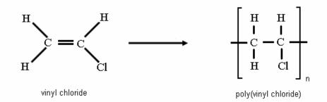
Figure 1: Structure of vinyl chloride monomer and polymer of polyvinyl chloride.
