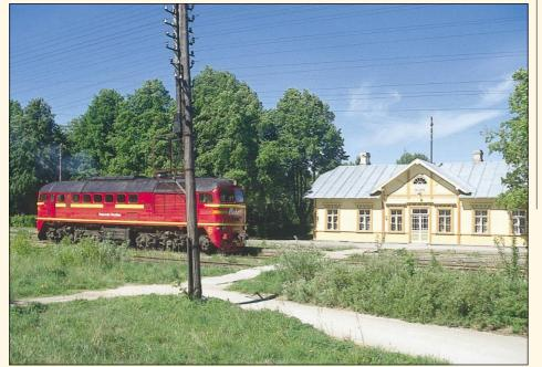
Left: Many industrial railways use Type TGM4 B-B diesel-hydraulic locos built by Lyudinovo from 1974 to a 15-yearold design. This loco, TGM4A-1134 belongs to Horizon Pulp and Paper (*Tselluloosi Ja Paberi*) and is seen at Kehra on 2 September 2002.
