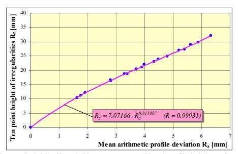
Fig. 6. The ten point height of irregularities R<sub>z</sub> versus mean arithmetic profile deviation R<sub>a</sub> for exponential mathematical model.
