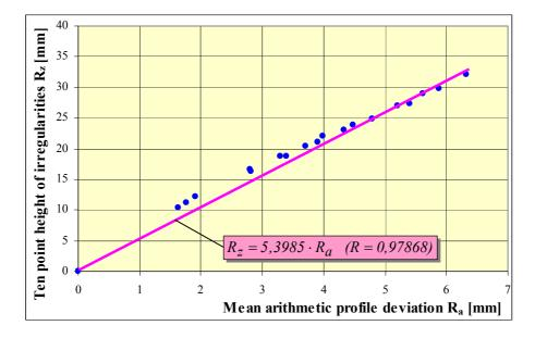
**Fig. 5.** The ten point height of irregularities R<sub>z</sub> versus mean arithmetic profile deviation R<sub>a</sub> for linear mathematical model.
