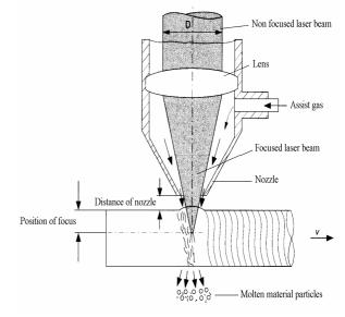
Fig. 1. Gas assisting laser cutting.
