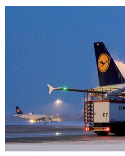
Use of snow ploughs, if necessary also chemical deicing agents based on formates; the waste water from deicing is caught in gutters and fed to the sewage plant in nearby Eitting.
