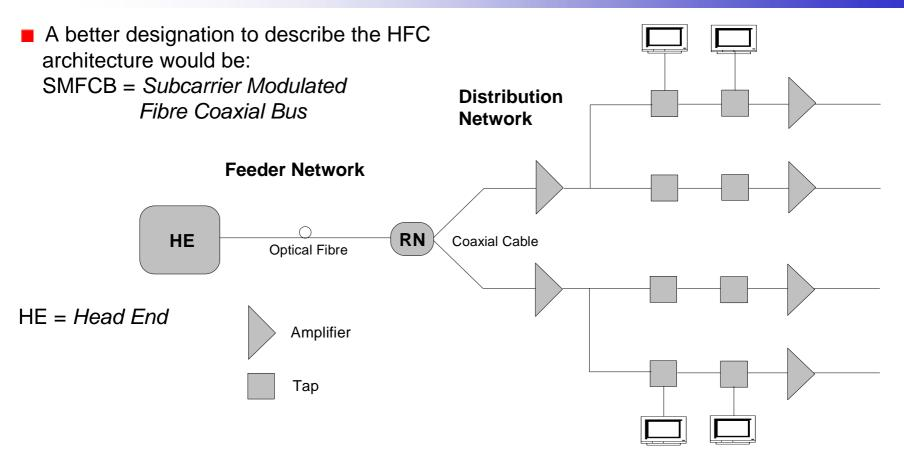
The feeder network uses the signal of a laser with SCM (*Sub Carrier Multiplexing*).
