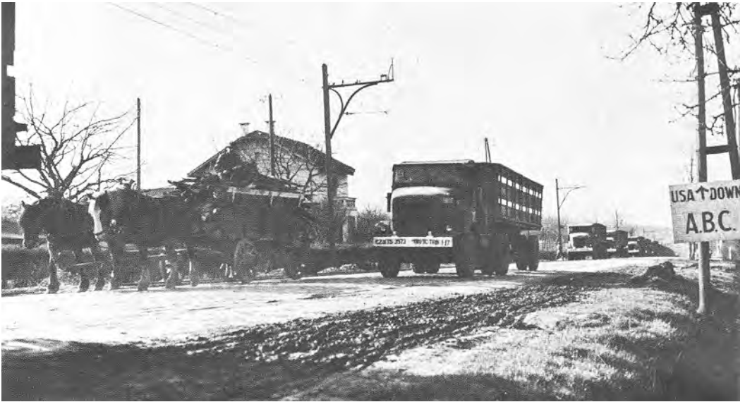
TRUCK TRACTORS, 5-TON, HAULING 10-TON SEMITRAILERS to Liège over the ABC Route, March 1945.
