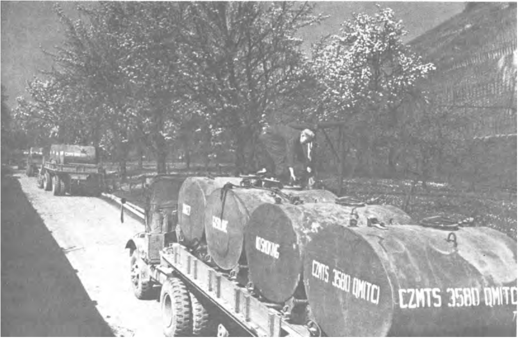
FOUR 750-GALLON SKID TANKS mounted on 10-ton semitrailers used for transporting gasoline in bulk.
