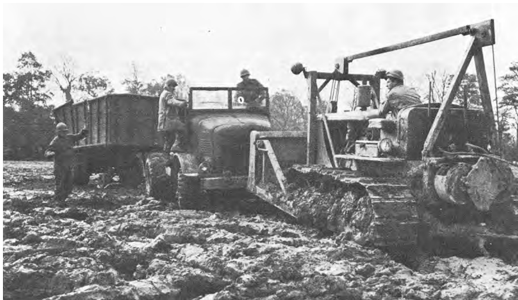
TRUCK-TRACTOR AND SEMITRAILER STUCK IN THICK MUD are pulled out by a D-7 tractor, Cherbourg area.
