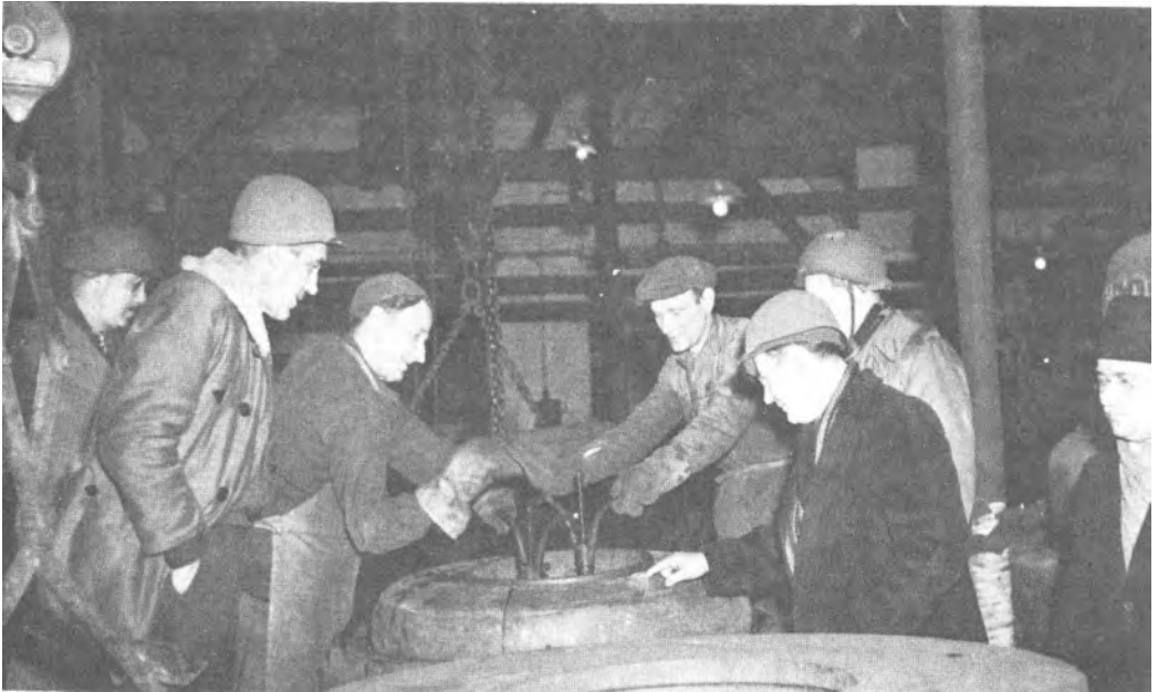
BELGIAN WORKERS IN A RUBBER PLANT, Liège . Members of U.S. rubber industry watch as a tire is removed from a mold.
