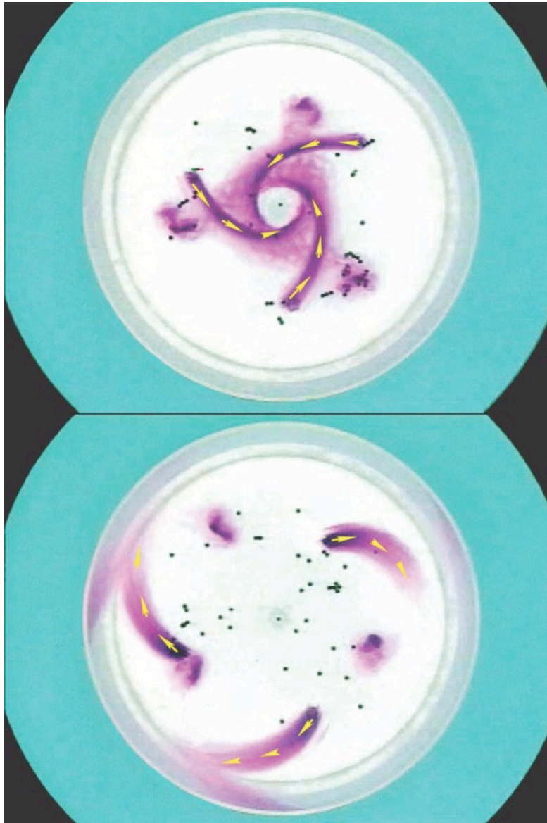
Figure 4: To carry out the experiment we first very slightly reduce (by 10% max) the rate of rotation of the turntable. Because of the inertia of the turning fluid, it continues to spin at its original speed and so moves relative to the tank: permanganate streaks are pulled around not in circles as one might initially expect, but rather inward turning, anticlockwise spirals, as can be seen in the top panel. A beautiful symmetric pattern is remarkably easy to achieve. This is analogous to the near-surface flow in a low pressure system, as can be seen by comparing with Fig.2 (see low pressure system). To visualize the flow at the upper surface, we can float a few paper dots on the surface (black dots are the most visible in this application). We observe circular, rather than spiraling, motion. To create an analogy of a high pressure system we now simply increase the speed of the turntable by 10% or so (back up to, roughly, its original speed). We observe the dye streaks on the bottom reversing and, over time, spiraling clockwise and outwards, as can be seen in the lower panel in this figure. This should be compared to the pattern of surface winds that can be seen in the high pressure system marked in Fig.2. From Marshall and Plumb (2007).
